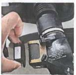
Step 4: Ensure that the fuel tag is within one inch of the hose module and begin fueling.
