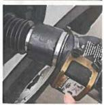
Step 3: Insert the nozzle in the fuel tank. Press the green button on the hose module.
